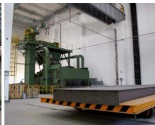
The steel in the VTC205 is shot blasted to create a fantastic painting surface
