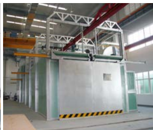
The VTC205 is painted and temperature cured eliminate corrosion
